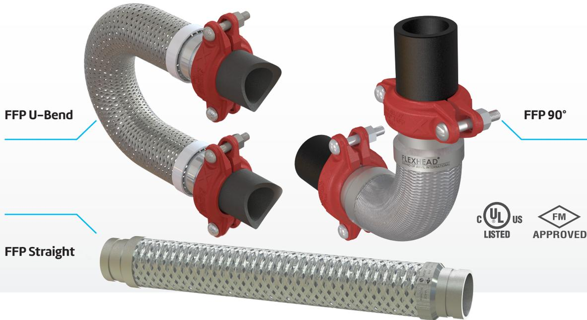
Flexhead® Flexible Pipe (FFP) products are stainless steel hoses and available with SLT coupling connections. Available in lengths of 24" (bends up to 90°) and 48" (bends up to 180°) with OD of 2", 2 1/2", 3" and 4". Pressure rating for 2", 2 1/2", and 3" is 300PSI and 4" at 250PSI. An easy, cost effective, and a quickway to connect pipes at odd angles or to reduce the number of couplings and fittings required.
